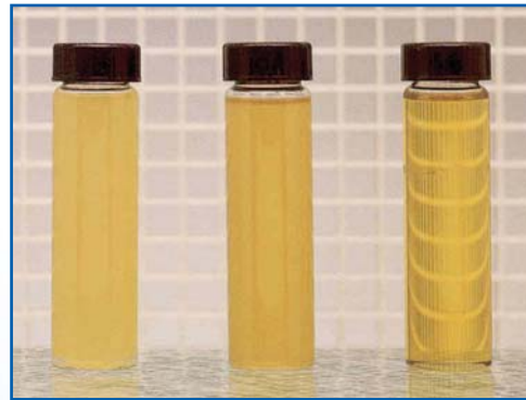
Free water removal in typical turbine oil: bright clear aspect shows absence of free water
