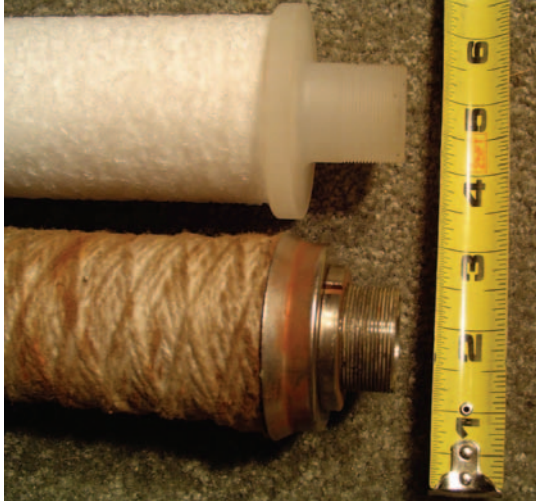
Figure 2 – End-cap and connector of Hydro-Guard filter element (top) and the string-wound filters
